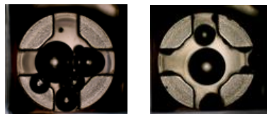
Figure 4. Dispensing 2.5 - 3 mL of cold Matrigel per block in the LoadingPlate for rapid loading of Matrigel on the pillar plate.
